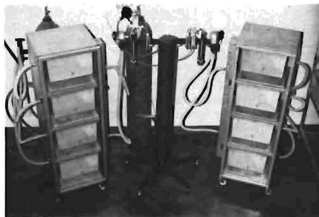
Fig. 3 Inhalation chambers with central gas metering and mixing apparatus.
