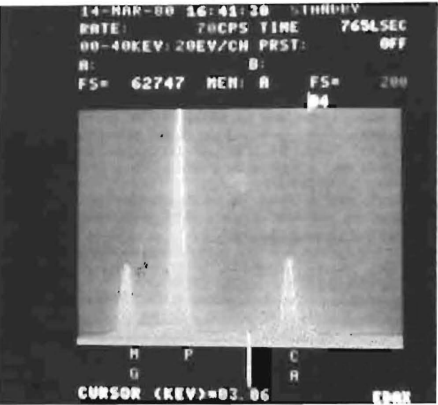
Fig. 6. X-ray energy dispersive analysis display of the entire area imaged in Fig. 5. The P peak is due to the presence of both struvite and hydroxyapatite, while Mg is due to the former only and Ca to the latter only.
