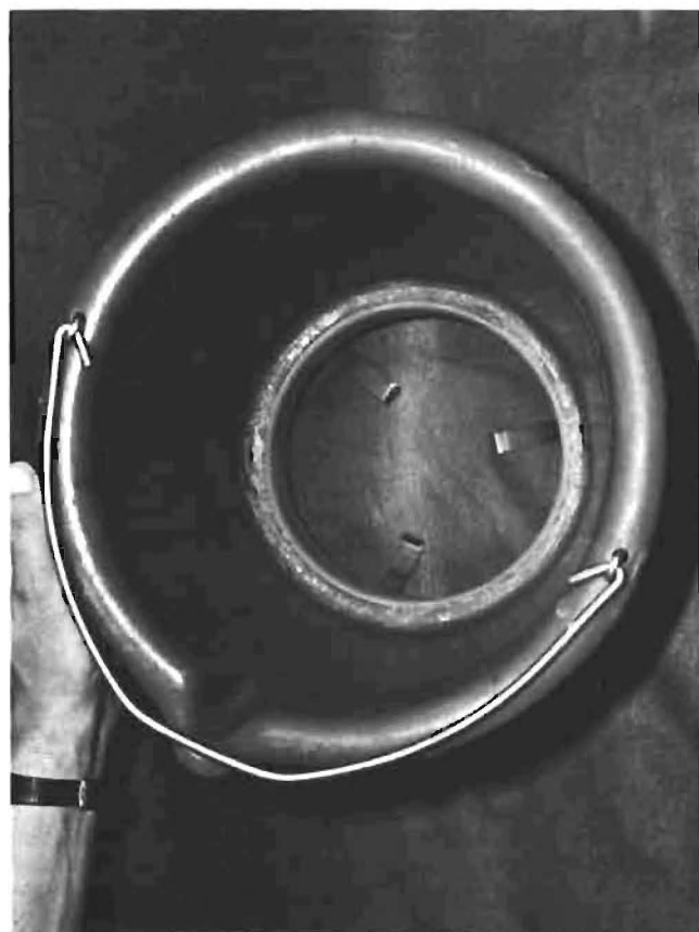
Fig. 3 Special bucket with a machined plastic pipe inserted in the base to allow the sieve to be placed in it for sieving; Upper and lower views (Helena Smit, University of Pretoria)
