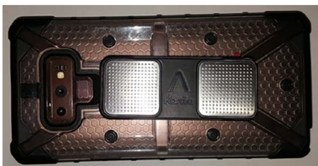
Figure 1: Alivecor KardiaMobile device secured to the back of a smartphone using the provided holder
