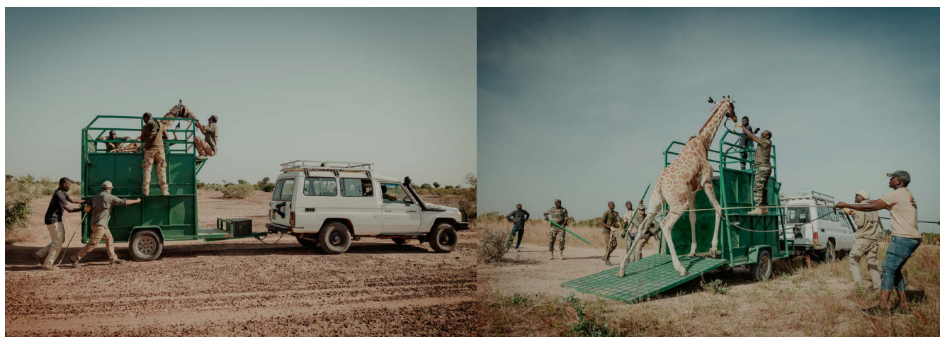
Figure 1: Field chariot. A modified horsebox, it was made fit for purpose with the addition of the following: standing rails along each side to allow access to the giraffe and enable staff to travel with the animal. Rear door modified to ramp (from swing) with mesh grating added for efficient loading and to reduce slipping. Modified, simplified and more robust door closure latches. Additional guard railings at giraffe head/neck height on sides and front to better protect the animal when moving. Two horizontal rear removable bars which allow the internal dimensions to be reduced depending on giraffe size to stop the animal turning around in the chariot and to give better lateral stability. A variable height and "distance-from-front" padded front bar to give the giraffe additional stability whilst reducing chance of chest injury, and to reduce the ability for giraffe to turn around in the crate. A strengthened towing arm with integrated tool kit, better able to handle rugged terrain and with all the necessary tools in case of puncture. Contact GCF for schematics.
