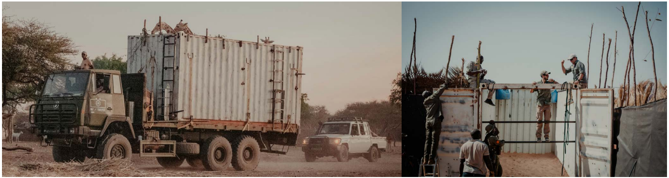
Figure 2: Transportation crate. A modified shipping container, it was made fit for purpose with the addition of the following: Roof removed. Door closure modified to have removable top cross strut to allow loading of animals, but which retains structural integrity and strength during transport. All sharp edges smoothed with grinder. Painted white to reflect heat. External ladders welded onto crate to provide access to top of crate for feeding and monitoring. Wooden pole attachment points. Short wooden poles for hanging browse. Wall mounted cut 200 L drums for water during transport (edges made smooth and a cutout to make access more comfortable for giraffe). Two rear horizontal poles to enable the giraffe to be secured whilst the doors are being closed/opened and the cross-strut replaced (also short pole guides externally, poles also locked in place by pins attached to wall of crate). Two short vertical rear poles at each side of door from which a dual cross line is strung to hang and pull a curtain, used when loading to prevent escape whilst the rear poles are fitted and the door secured.
