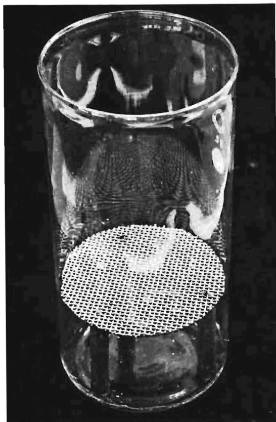
Fig. 2. — Glass jar with a false floor of wire mesh.
